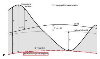
Figure 10: Possible scenarios of computing the topographic gravity correction for a height reference surface represented by (a) the geoid, (b) the geometric reference surface and (c) the Bjerhammar sphere/ellipsoid. Used notation: h the geometric height, H the physical height, N the geoidal height and D the (constant) depth of the Bjerhammar sphere/ellipsoid.
