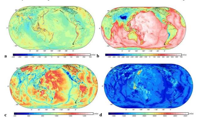
Figure 1: Global gravity: (a) free-air, (b) Bouguer, (c) mantle and (d) sub-lithosphere mantle.
