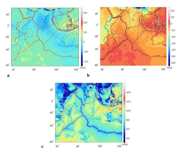
Figure 2: Gravity of the Indian Ocean: (a) free-air, (b) Bouguer and (c) mantle gravity data.
