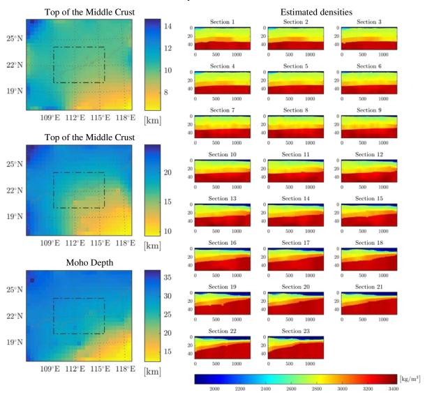
Figure 12: Estimated GIGJ model under the JUNO detector by the Bayesian inversion of GOCE data. Discontinuity surfaces on the left, density distribution on the right. Note that the top of the Upper Crust (i.e., the basement) is not estimated. Note also that the sections are numbered from North (1) to South (23), and cut the model from West to East.
